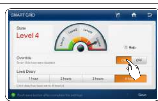
[Encender Override (Anular), Apagar Smart Grid]
