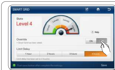
[Apagar Override (Anular), Encender Smart Grid]
