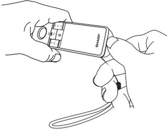
Figure 3: Pull the handle rope with your middle and index fingers and use your thumb to open the battery cover.
